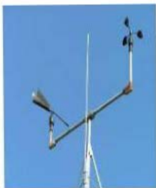
Fig. 1.17 a A rotating cup anemometer
