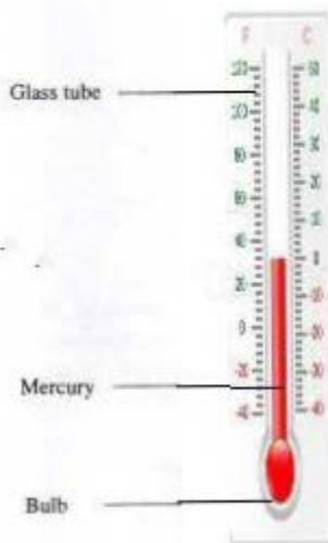
Fig. 1.14 A simple thermometer
